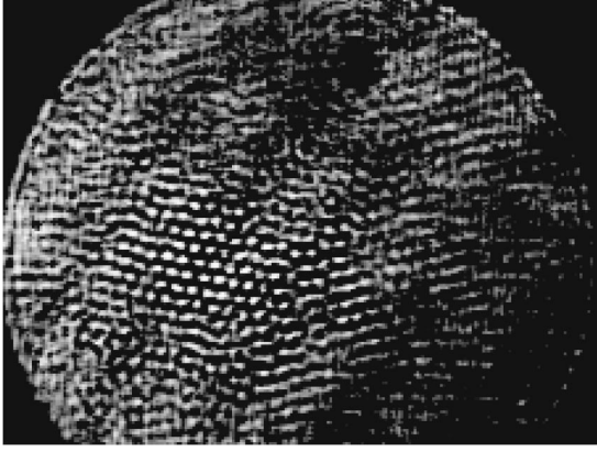
FIG. 7. Experimental snapshot of a pattern close to threshold, without control. The hexagonal pattern starts to grow locally, where the nonlinearity is most sensitive.
